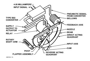
Figure 7. Schematic Diagram of Type 3582i Positioner
