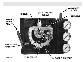
Figure 4. Type 3582 Pneumatic Valve Positioner Mechanism
