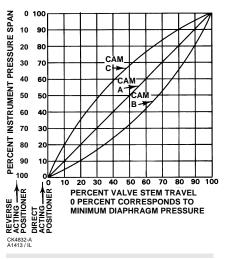
Figure 8. Instrument Pressure Versus Valve Travel
