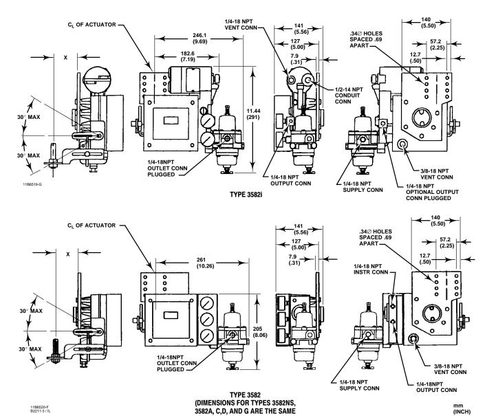
Figure 11. Valve Positioner Dimensions and Connections
