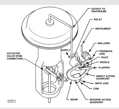
Figure 6. Schematic Diagram of 3582 Series Positioner
