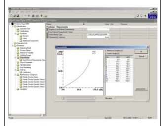
Fig. 5 · TROVIS-VIEW Configuration and Operator Interface, dialog box for user-defined characteristic
