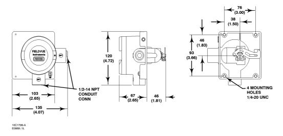
**TYPE DVC6035 ROTARY ACTUATOR SHAFT MOUNTING**
