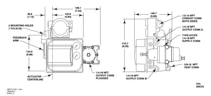
Figure 12. Dimensions for Type DVC6010 Digital Valve Controller with Integrally Mounted Filter Regulator
