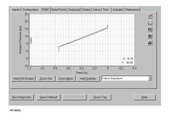
Figure 6. The Valve Signature Display
