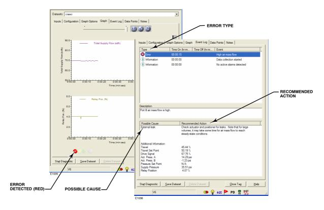
Figure 4. One-Button Sweep—Air Mass Flow Diagnostic
