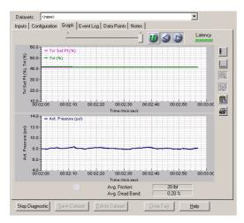
Figure 5. Valve Friction and Deadband Analysis
