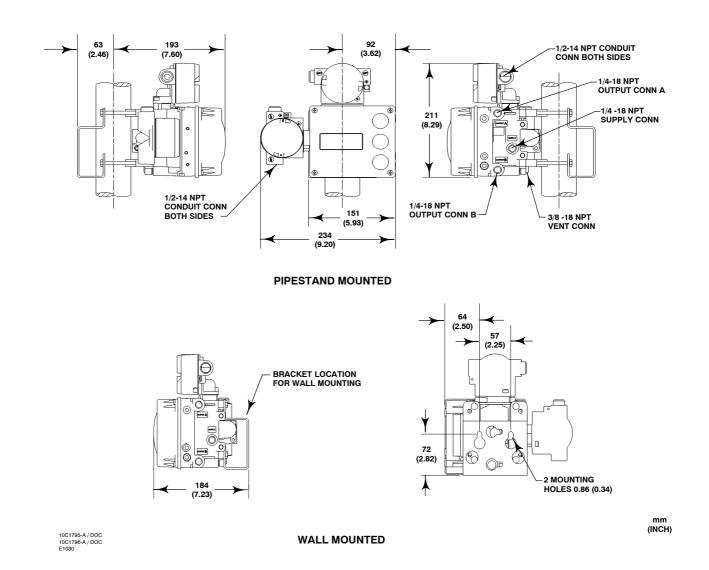
Figure 15. Dimensions for Remote-Mounted Instruments—Type DVC6005 Base Unit
